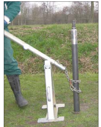
Pulling out the first gouge with the rod puller extension
